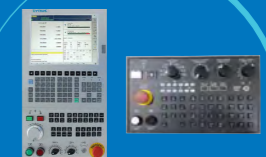
System OEM Machine Operation Panel
