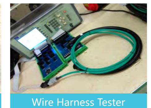
Various interface test boards
