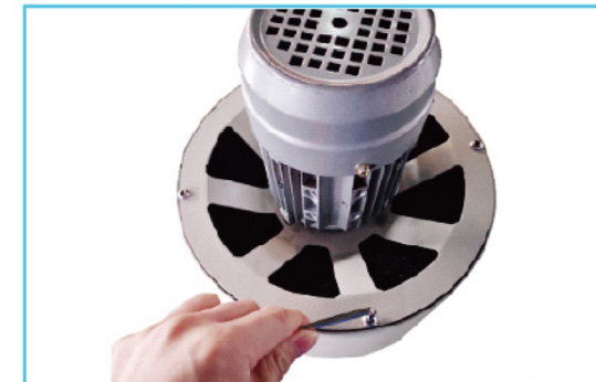
Unscrew the Allen screws and remove the secondary filter wool for replacement.
